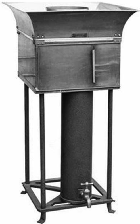
Figure 2: Rain gauge made by Julien P. Friez & Sons
